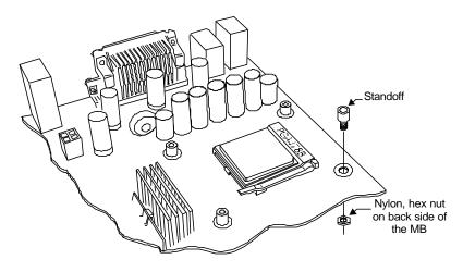
6. Re-install the MB inside the case.
