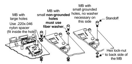
Install standoff in each one of the four holes surrounding the socket. Keep the standoff & washer centered over the MB holes, and secure with hex lock nuts on backside of the MB.
